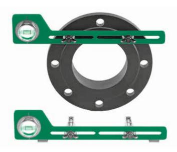
(fixing by slip-in pivots) this spirit level has adjustable slip-in pivots which fit flange bolt holes of various diameters. The adjustable water-level is surrounded by a scale. The scale has both: Degree and inclination-percentage markings. Any angle of degree or inclination can easily be set and read without the need for additional calculation. In this way flanges can be aligned with great accuracy. Material: Anodized aluminium.
