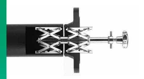
this model has two independent expanding clamps, allowing coaxial alignment of two hollow cylindrical components of different diameters. The bottom expanding clamp is inserted and clamped in the pipe by means of the knob. Then the other part (e.g. a flange) is placed over the top expanding clamp and clamped by means of the hand-bar. Compared with model 3a. This model is specially suited for heavy parts. Automatic diameter compensation.
