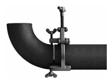
for exact centering and clamping of pipes without restriction in length. Also for curved tubes, flanges, T-shaped and other parts to pipes. The assembly of pipe-systems can be practised by only one pipefitter. Welding parts are accessible from all directions. Microadjustment device by wing-screw. To avoid corrosion we recommend stainless steel type.
