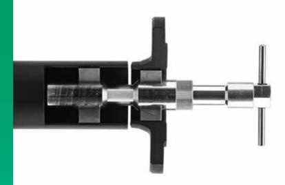
for guick and accurate alignment and clamping of flanges, nozzles, short pipe sections to pipes and cylindrical tanks. Wedge shaped clamps provide automatic compensation even for parts with greatly differing diameters.
