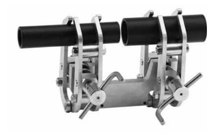
for quick and accurate alignment of pipes of **equal or differing diameters** on a common center line. **Automatic diameter compensation.** There's no need to make additional adjustments. All part stay easily accessible for welding.
